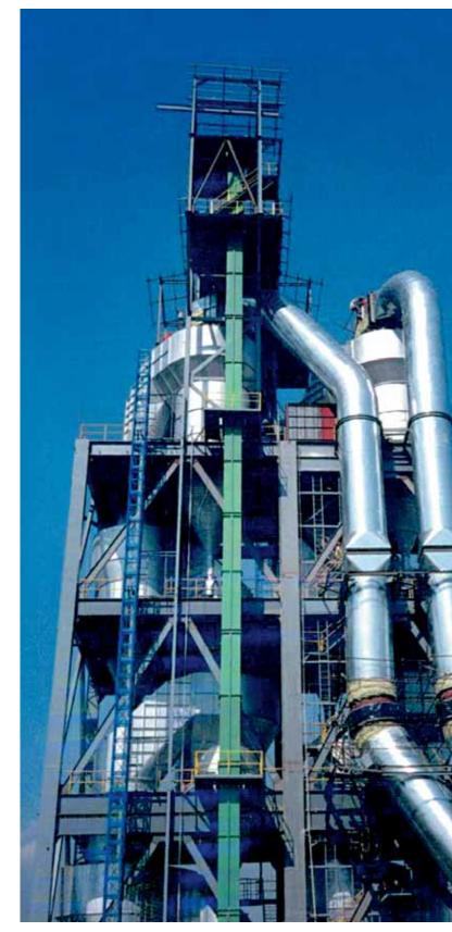
Belt Bucket Elevator for Pre-Heater Feeding
