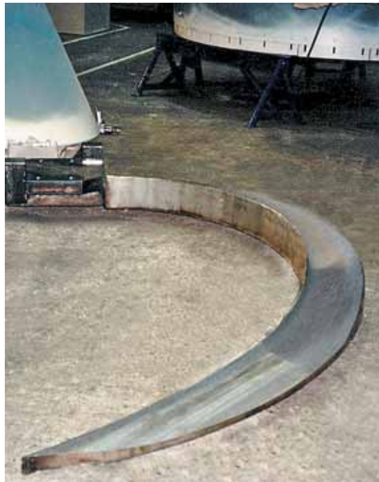
CENTREX™ discharge arm for internal drive
