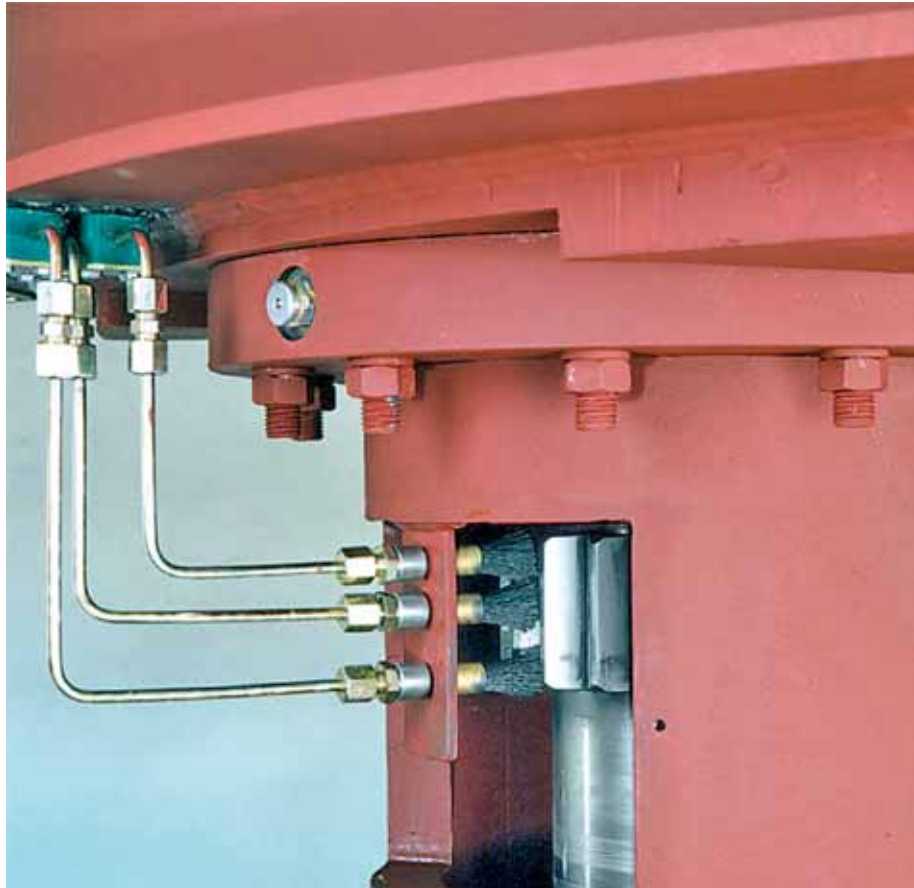
Two separate lubrication lines: one to lubricate the gear of the slewing ring,
