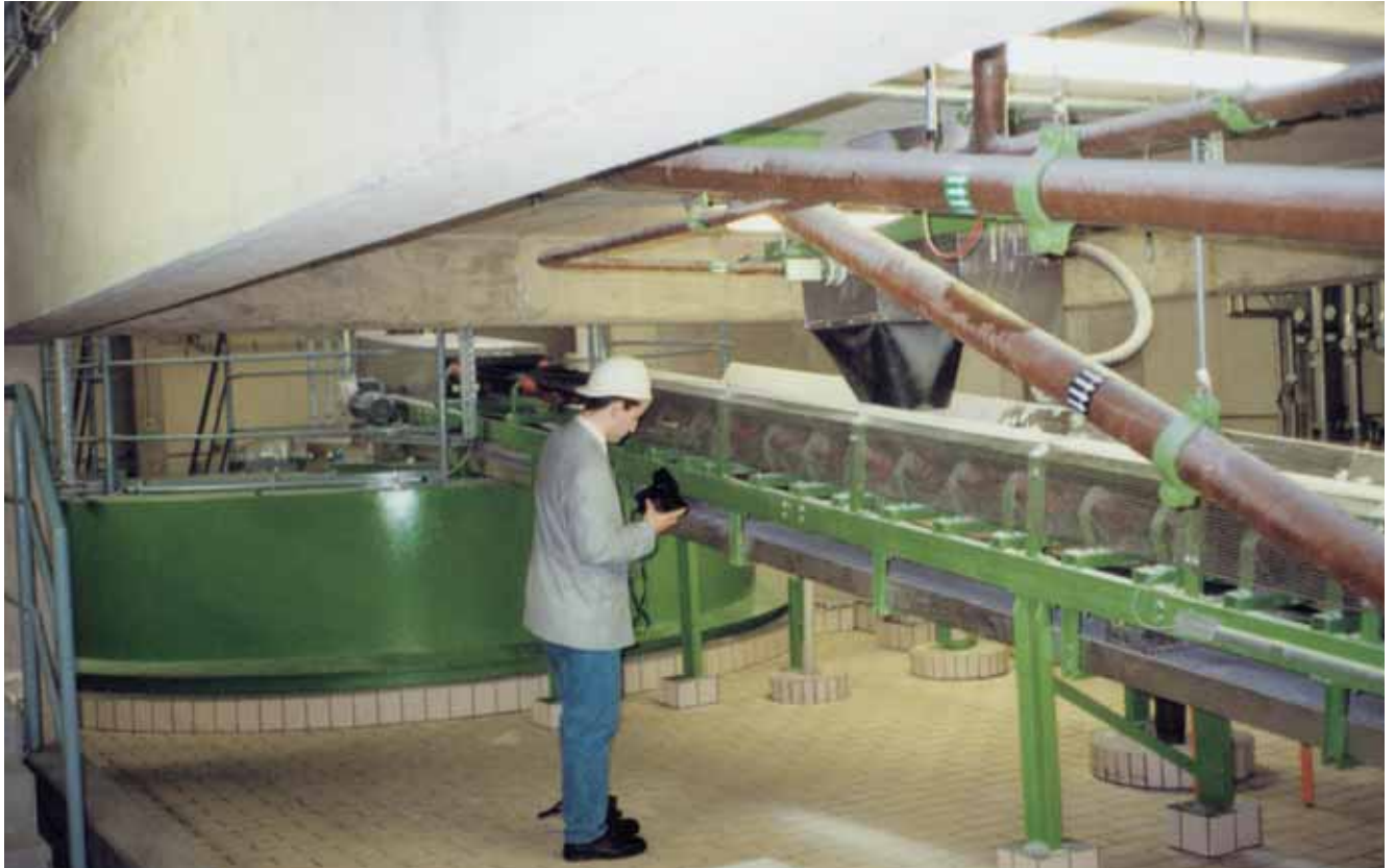
CENTREX™ - Feeding of FGD Gypsum to silo
