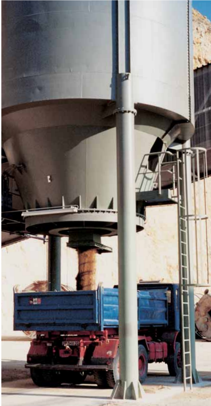
CENTREX™ with internal drive. Discharge from a steel plate silo with truck loading
