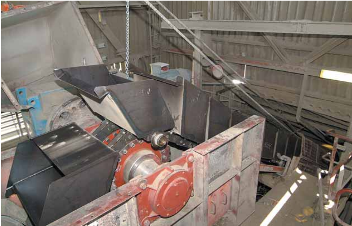
Installation of new bucket strand
