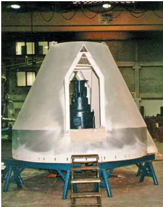
Ready assembled CTX-I 5000, view into the support/maintenance arm, onto the planetary drive unit
