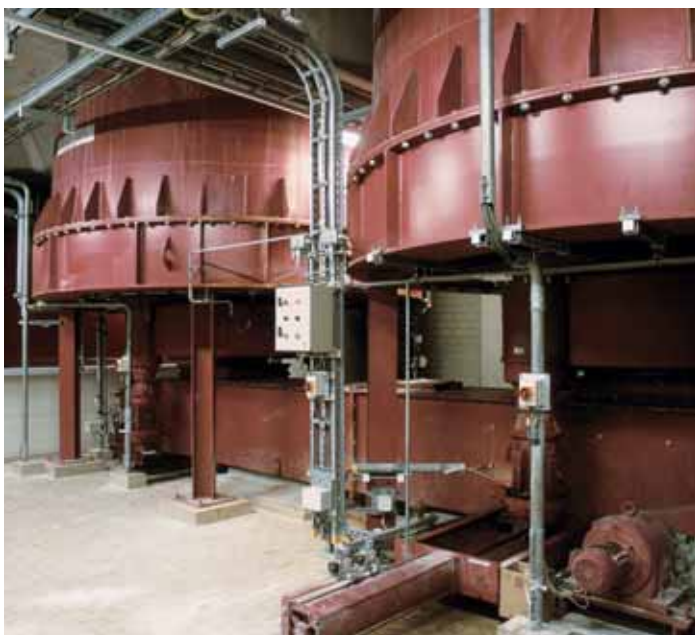
CENTREX™ type CTX-A with external drive for FGD Gypsum
